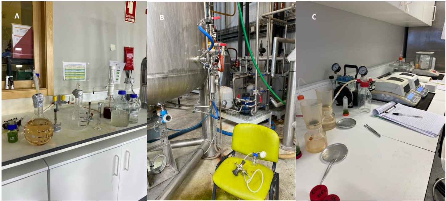
Figure 6: A: Inoculation of new cultivations, B: sampling of heterotrophic Chlorella for inoculation, and C: measurement of sample's dry weight.
